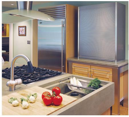
The concrete sink for herbs incrementally increases from 2- to 4-inches deep, which accommodates a pot filler faucet and provides a visual and functional connection to the clients' garden.
